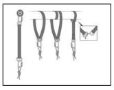
It offers several configurations for setting up an anchorage directly on an anchor or around a suitable structure.
