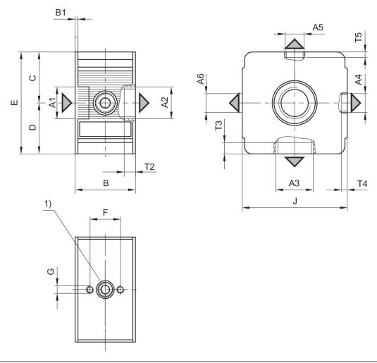
A1 = input A2 = output A3 = output A4 = output A5 = output A6 = output 1) hole pattern for mechanical vacuum/pressure switch
