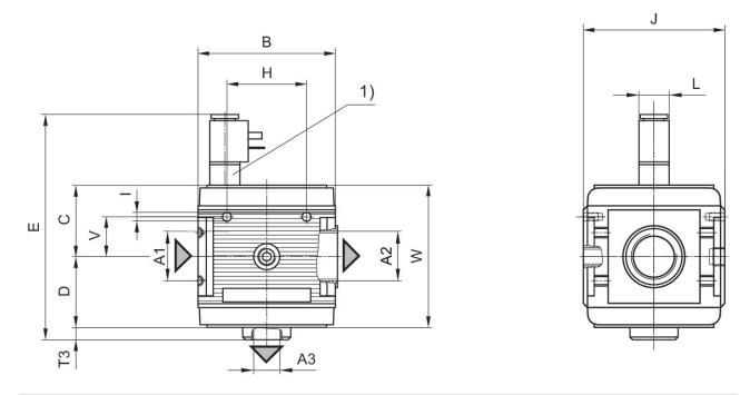
A1 = input A2 = output A3 = ventilation port 1) electrically operated
