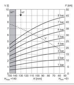
V = volume H = height H\* = recommended operating height for vibration isolation H\*\* = use permitted only upon approval by AVENTICS 1 kN = 1000 N
